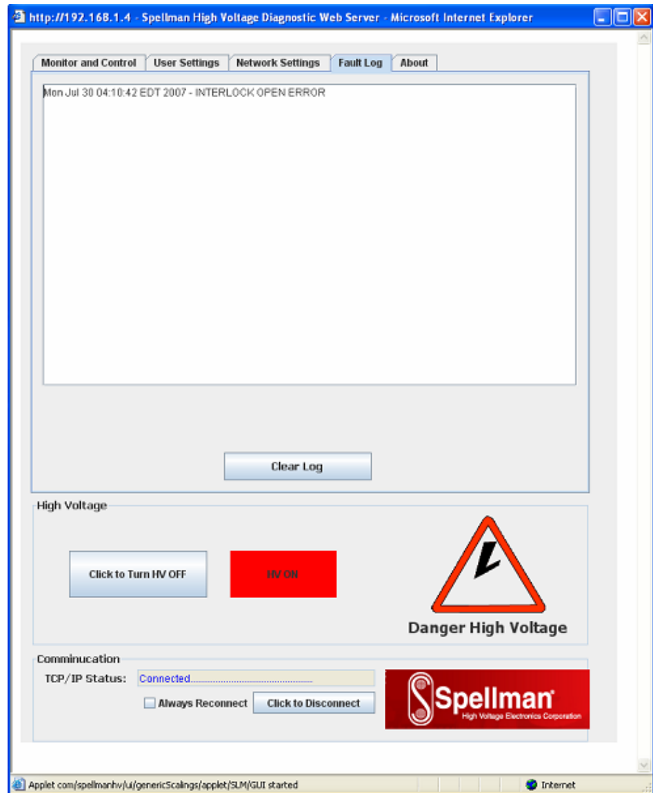
Figure 14 – Fault log Fault log displays faults with their date and time.
