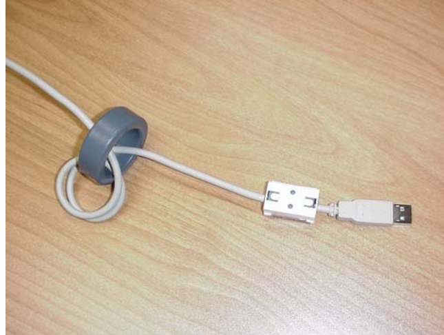
Figure 8 - Example of a USB Cable Using Ferrites
